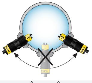
The flow switch tips have a thin plastic wall which may be damaged if dropped or installed improperly.
