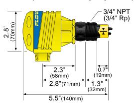
**Set Points:** The AT1\_-\_63\_ series liquid flow switch set point is factory calibrated to 0.2 fps and the AG1\_-\_36\_ series gas flow switch is set to 10 fps. To convert feet/sec to GPM, please refer to the chart below.
